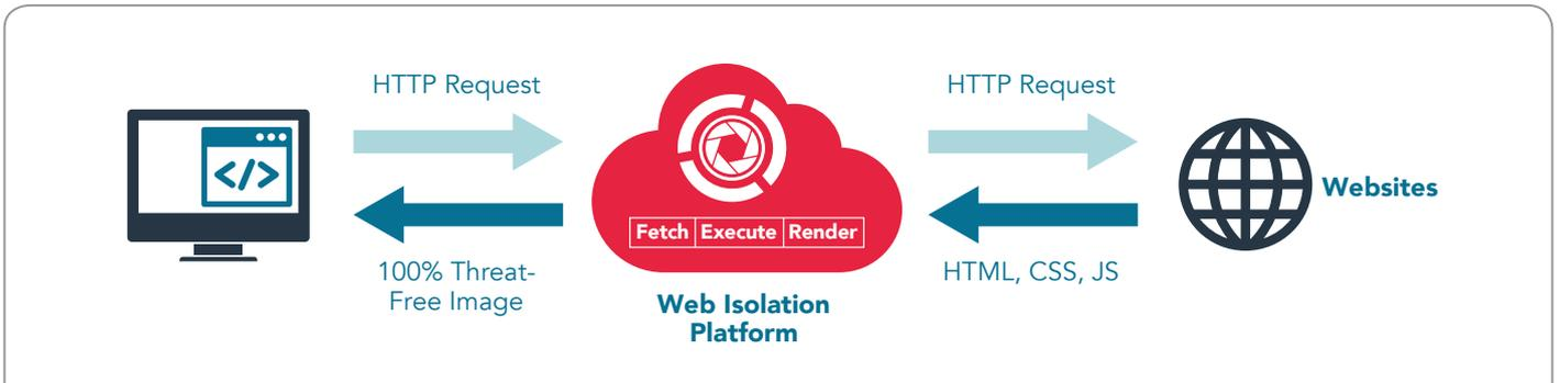
All web content are executed and rendered in a secure and remote environment. In this way, web isolation prevents malicious web codes from ever reaching your network and end user devices. For further protection, each end user's Web session is confined to a virtual browser that is disposed at the end of the session, thus eliminating malware persistency.
