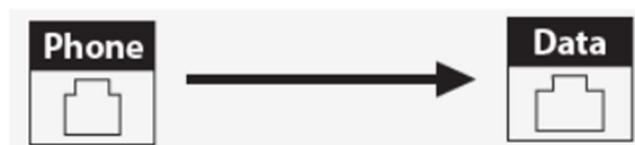
If your socket plate only has a phone port, and structured cabling has already been installed at your home using at least a Cat5e Ethernet cable, you can convert the socket plate from a phone port to a data port.
