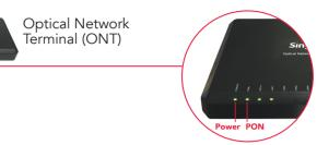
Use RJ45 Ethernet cable to connect LAN 1 port on the ONT to the blue Internet port of the
