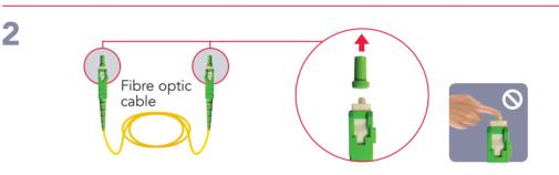
Remove both green caps from the fibre optic cable. Do not touch the tip of the cable as dust and fingerprints may cause interference with the connection and affect your internet speed. **Note: A fibre optic cable is made up of glass – do not stretch, tie or bend sharply.**
