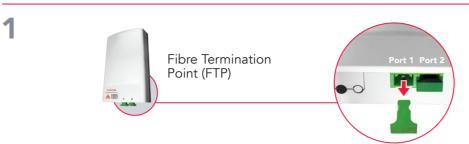
Unplug the green plastic cover from port 1 on the Fibre Termination Point (FTP). Note: FTP can be commonly found near your household distribution board (DB box) or near your TV point.
