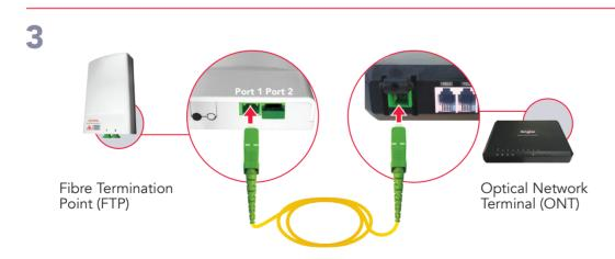
Connect the fibre optic cable from port 1 of the FTP to the Passive Optical Network (PON) port located at the back of the Optical Network Terminal (ONT).
